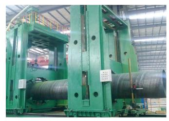
The Lincoln Welder uses an advanced double submerged-arc welding technique
